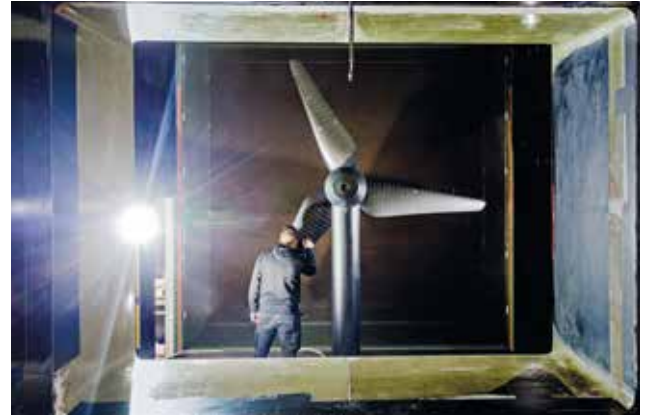
Optimization of wind turbines in the wind tunnel at TU Berlin
